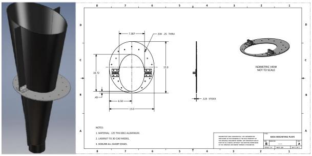
The base, funnel, and base (to floor) mounting plate fit together making assembly a snap, and result in a rock-solid permanent installation.
