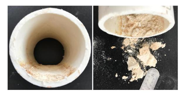
Then, after 5 years of use the drain pipes were "fully removed" again. As you can see in the photo below there was almost no increase in the accumulation despite having been in use for over twice as long. As was the case 5 years earlier, the residue was viscous but flowable. The photos below were taken a few days after removal to let the flowable residue dry enough to set up so the photos could be taken.
